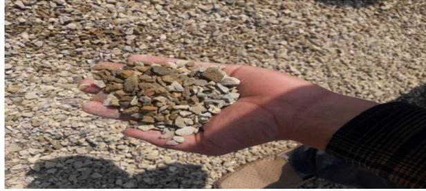
Figure.2 Coarse Aggregates
