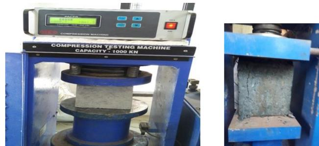
*Figure.3 Setup for Compressive strength*
