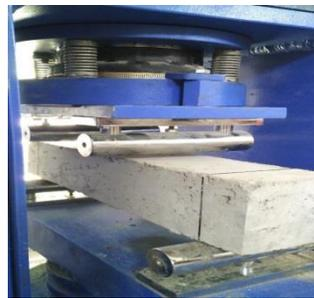
Figure.5 Flexure Strength Test
