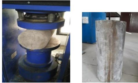
Figure.4 Setup for Split Tensile Strength
